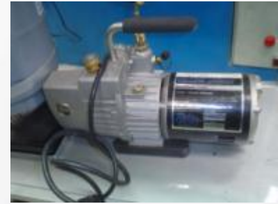
VACUUM PUMP WITH GAUGE METER WITH AN ACCURACY IN MICRONS
