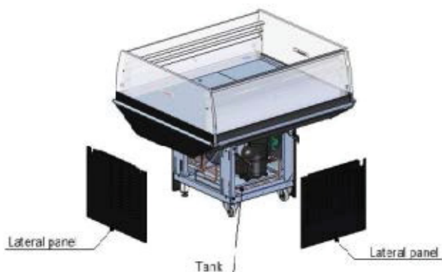
Fig. 15 Removing condensating unit panels
