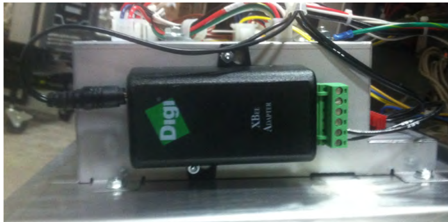
Figure 6-4 Securing Radio to Control
