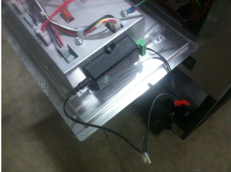
Figure 6-2 Sliding Radio Module on to Studs
