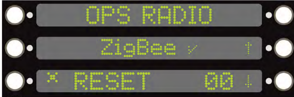
Figure 6-17 Reset/Unjoin Command Display
