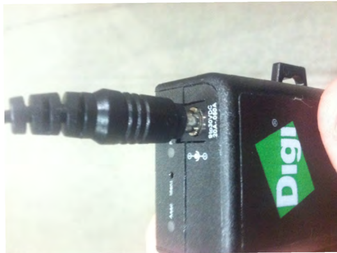
Figure 6-3 Attaching Connector to Radio
