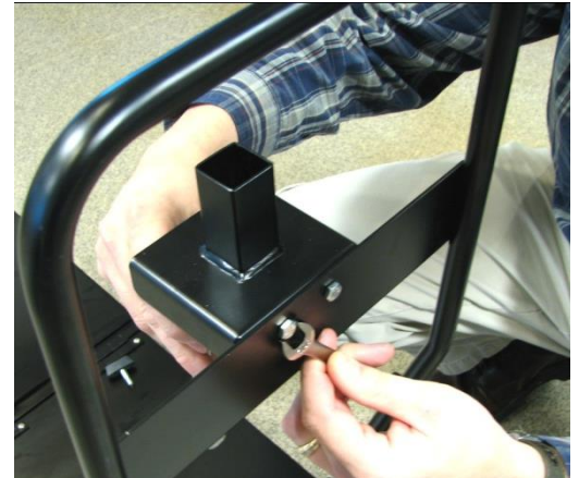
BOLT BRACKET TO HANDLE WITH BOLTS PROVIDED AND SLIDE PUMP AND TUBE ASSEMBLY THROUGH SQUARE TUBE AND INTO ROUND TUBE.
