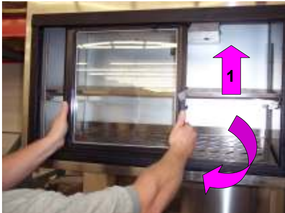
Figure 7. Removing Sliding Doors.
