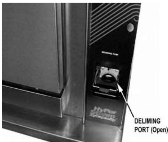
The De-Liming Port is at the Bottom of the Control Panel.
