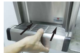
Install drip tray and cover.
