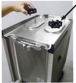
Install mixing impeller.
