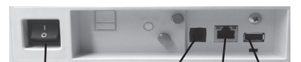
On/Off Power Switch Cash Drawer LAN (Ethernet Cable required to connect with PC) USB
