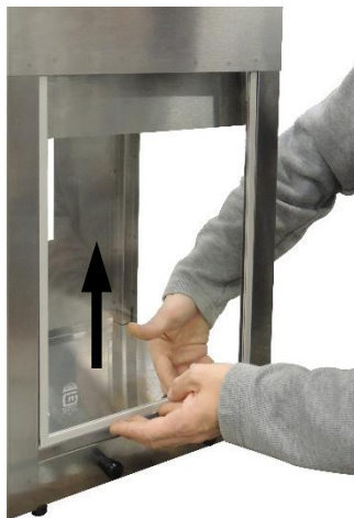
Figure A - Slide glass panel up under top ridge.
