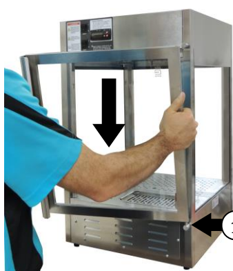
Step 9: Set bottom Door Pin into Hinge, then insert top pin thru hinge and fasten into door till snug.
