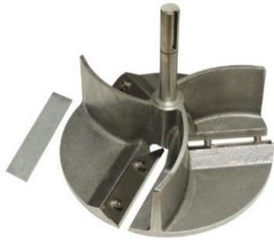
Shaver Head with Height Gauge .050" (thickness of a dime)
