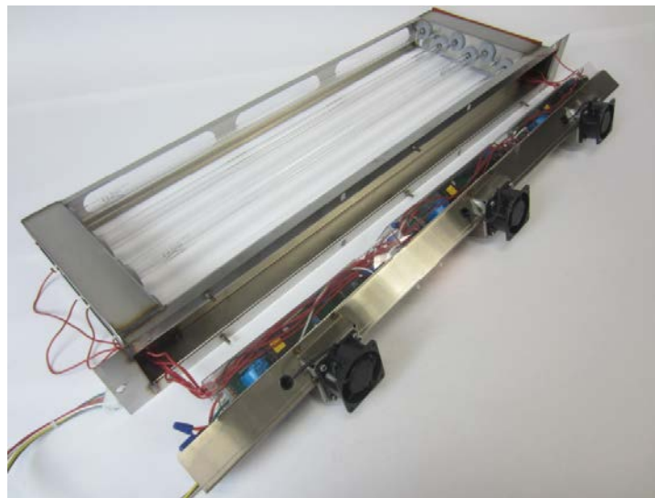
Figure 6-34-2 Ballast Raceway Removed from Module
