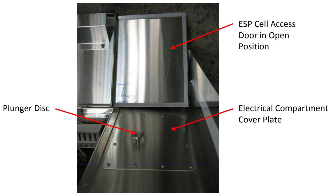
Figure 6-52-1 Access to the Electrical Compartment
