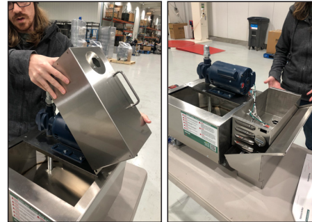
Step 3: Remove motor housing, pivot and rest the housing onto the caddy chute in order to take pressure off the wire casing.
