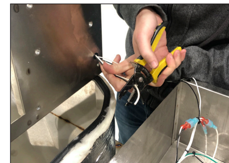
Step 13: Cut the heater belt wires and pull the wires back through the Caddy body.
