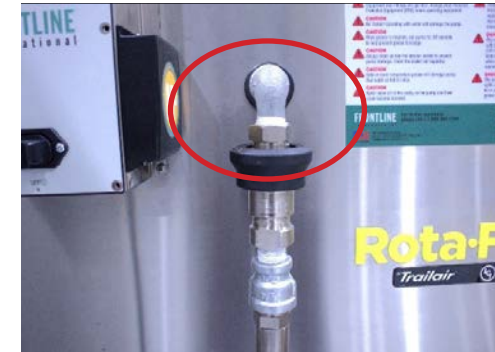
Step 1: Connect the caddy hose to the top of the caddy outlet. Then connect the hose to the tank inlet.
