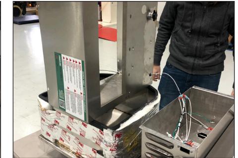
Step 12: ... and rest it on the Caddy body.
