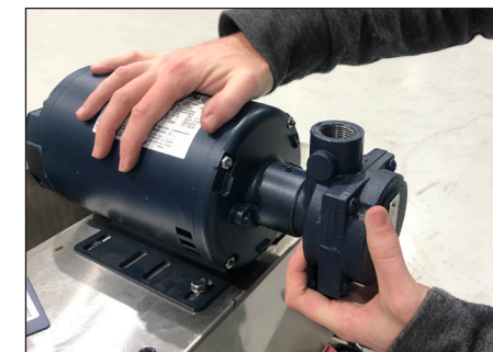
Step 13: You are now able to swap in the new Pump Head, replacing the old.
