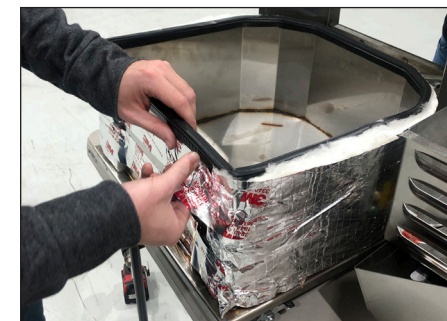
Step 14: Carefully remove the tape from the back of the bucket. If tape tears you will need to replace with heavy duty tape or duct tape when re-assembling.
