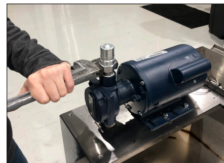
Step 4: Disconnect the quick disconnect from the top of the pump.
