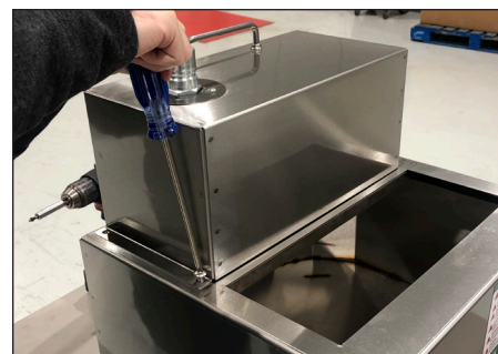
Step 18: Resecure the motor housing back to the caddy using the four screws. ■
