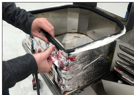
Step 22: Wrap the insulation back around the new belt. Secure with tape.
