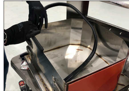
Step 21: Once springs are re-attached, re-secure the rubber gasket, starting at the mid-point of the FLAT backside of the Caddy assembly.
