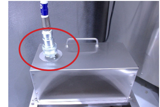
Step 2: Connect quick disconnect to top of motor housing.
