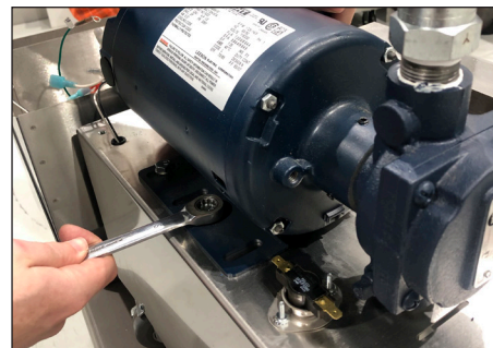
Step 27: Using the four bolts, reattach the motor to the caddy frame. ■
