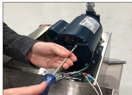
Step 5: Remove screws to open wire housing.
