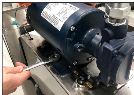
Step 8: Remove the four bolts that attach the motor to the caddy frame.
