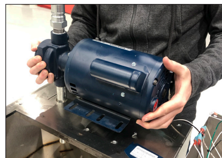
Step 9: Lift to remove motor. Turn motor 90° and set on the Caddy frame.
