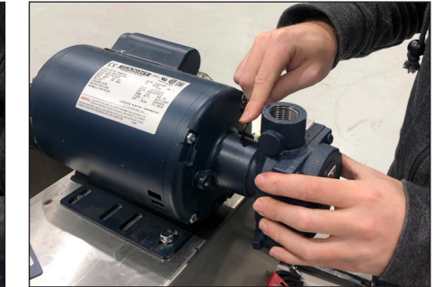
Step 12: Using an Allen wrench, loosen (don't remove) the three pins holding the pump head to the motor.
