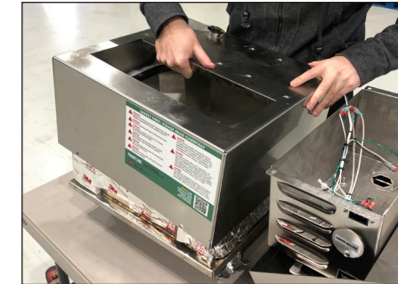
Step 11: Lift the bucket cover...
