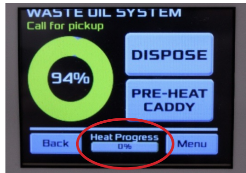
Step 2: The heating progress bar will show up on the bottom of the screen.
