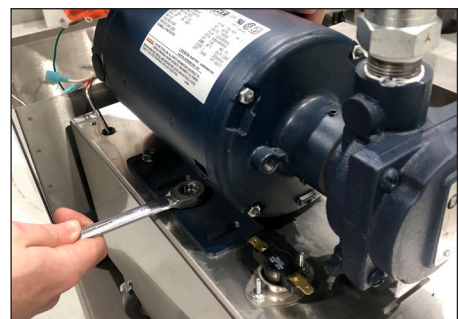
Step 16: Using the four bolts, reattach the motor to the caddy frame.
