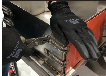
Step 20: Attach the springs.
