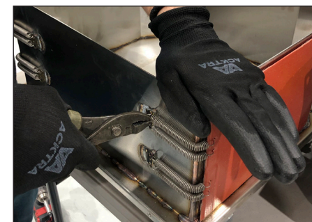
Step 17: Using pliers, unclip the springs, four on each side of the belt.
