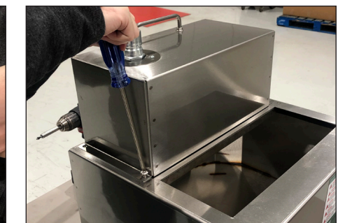
Step 18: Resecure the motor housing back to the caddy using the four screws. ■
