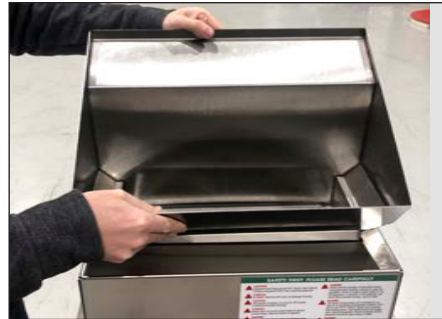
Step 1: Remove Grill Grease Caddy chute and basket and set to the right of the Caddy.
