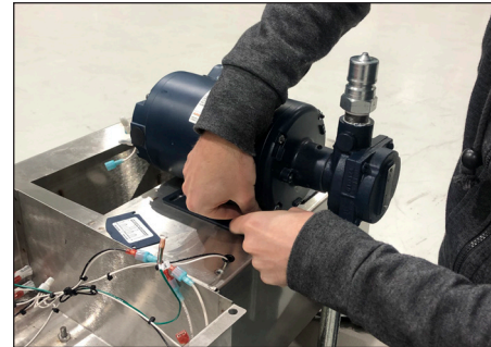
Step 10: Reinsert one bolt to create a stable work surface.
