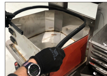
Step 16: Remove rubber seal from top of Caddy bucket assembly. Start at the middle of the flat front side.
