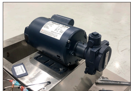
Step 12: You are now able to swap the new Motor and Pump Head assembly for old Motor and Pump.
