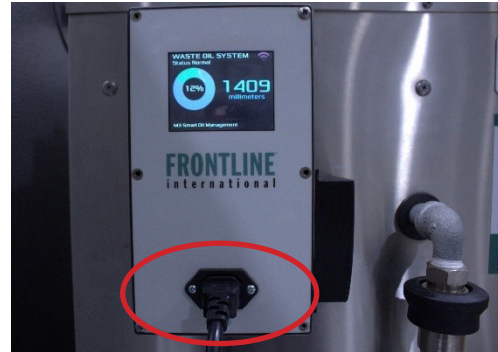
Step 2: Connect the power cord to the front of the control panel.
