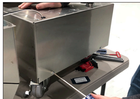
Step 24: Attach the body back to the bucket with the four screws.
