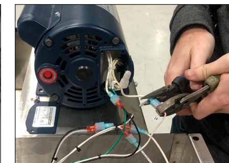
Step 17: Connect the wires back to the wiring harness terminals.
