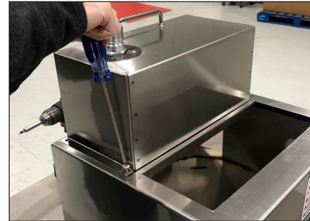
Step 2: Remove the four screws in the motor cover housing.
