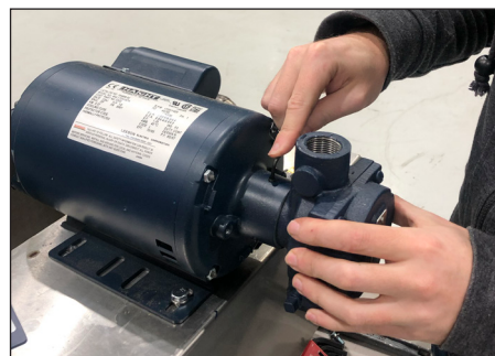
Step 12: Using an Allen wrench, loosen (don't remove) the three pins holding the pump head to the motor.
