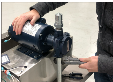
Step 11: Using a pipe wrench, remove the suck pipe from the bottom of the pump.
