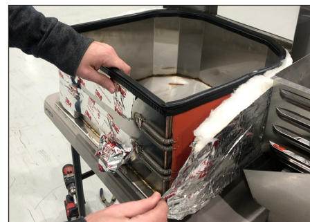
Step 15: Remove insulation to expose springs, setting insulation to the side.
