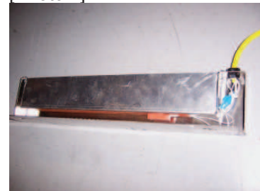
The tank heater is attached to the aluminum tank bottom and protected by a false bottom.
