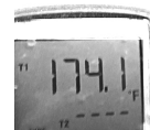
The pyrometer is showing a temperature within 5°F (3°C) of the cabinet display, an acceptable margin.
