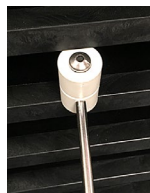
The button end of the probe is placed against the plate being measured.
