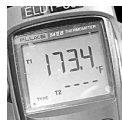
The pyrometer is showing a temperature within 5°F (3°C) of the cabinet display, an acceptable margin
