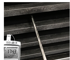
The temperature of all the heater plates are tested against the reading of the pyrometer.
