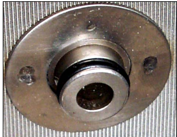
Inspect the filter screen O-ring.
