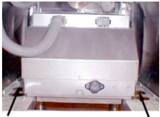
Location of screws securing contactor box to bottom frame
