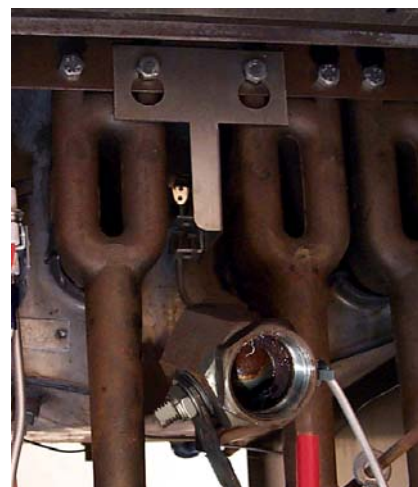
Remove drain valve handle and burners from fryer.
