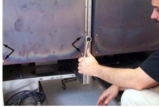
Removing bolts (arrows) securing flue to frypot.
