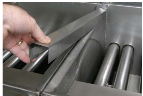
Removing the joiner strip.
