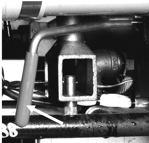
Push the red handle right to open drain valve. Oil will start to drain into filter pan.
