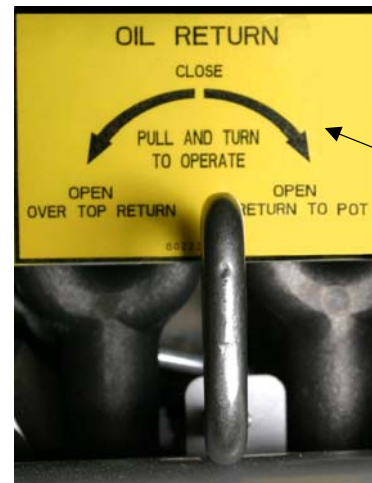
Pull and turn the oil return handle to open the oil return valve and activate the filter pump.
