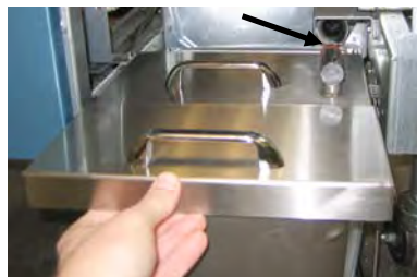
Figure 4: Place the lid on the pan and slide the oil pickup tube into the female suction receptacle.
