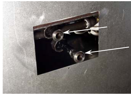
Figure 5. Oil return and rinse-line (where applicable) connections.
