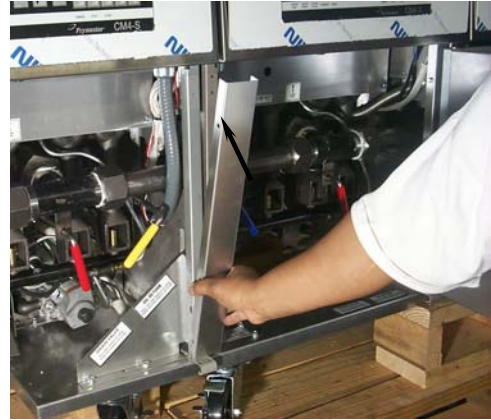
Figure 8. Installing front connecting post on connected fryer sections.
