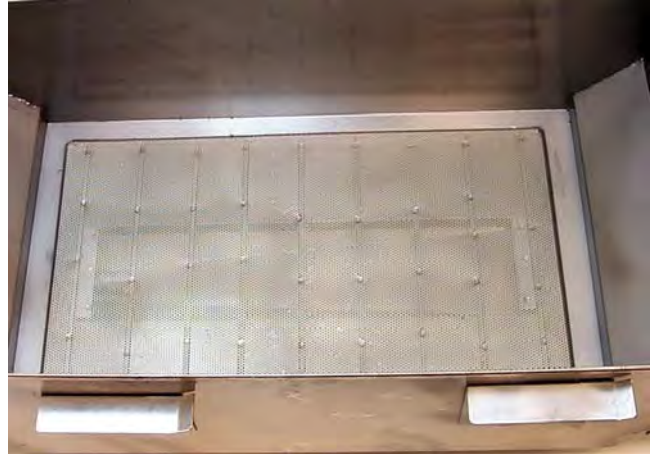
Support grid properly placed in filter pan.
