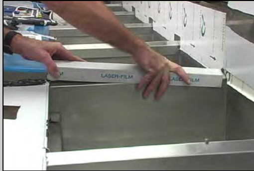
Figure 9: Place joiner strip which connects the frypots.
