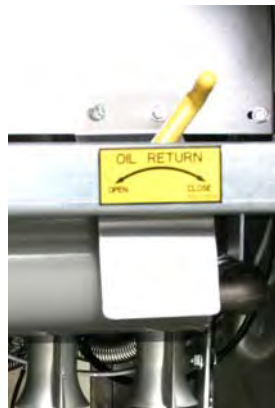
Return filtered oil to the frypot by rotating the yellow handle to open oil return valve.
