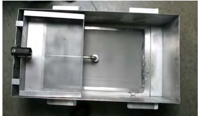
Crumb screen properly placed in filter pan.
