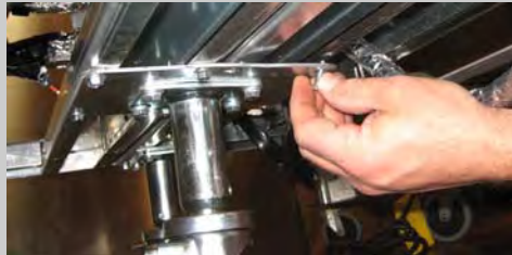
Figure 4: Align the fryers and secure the center mounting plate with bolts.
