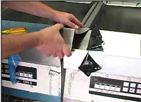
Figure 6: Attach strip joining the fryer sections. Install screws under the lower edge.
