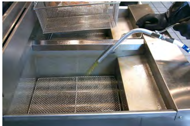
Use the optional wand to rinse debris from the frypot into the filter pan. Maintain a firm grip on the wand handle at all times.
