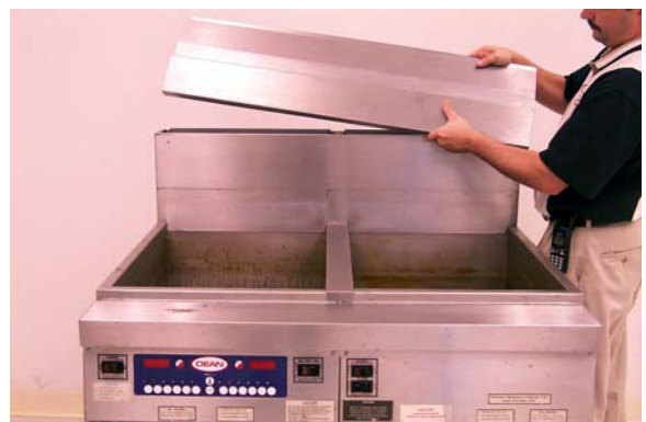
Removing the flue cap.
