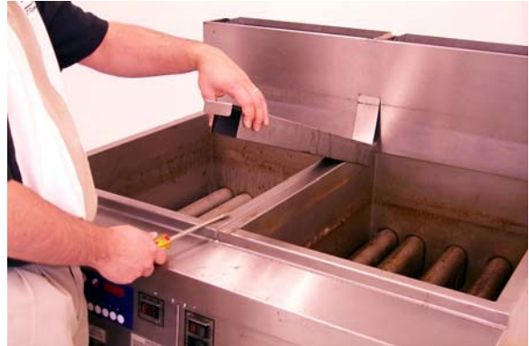
Removing capping strip.
