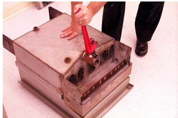
Removing drain valve from frypot.
