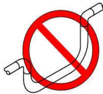
FIGURE 3. - Insufficient Condensate Trap
