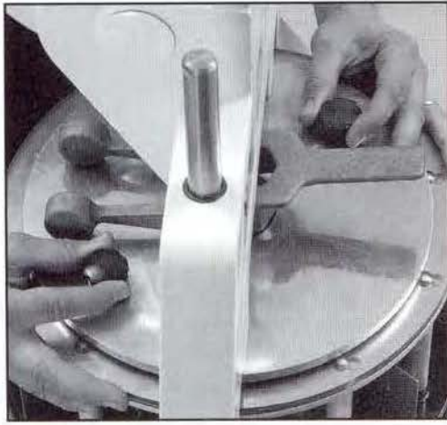
Figure 1: Remove pan, loosen completely both Black Knobs. ! WARNING: DO NOT DROP Divider Head Assembly as damage may occur!
