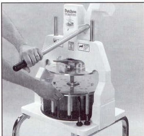
Figure 3: While holding Handle down with one hand, with the other hand rotate Head Assembly? turn until Head Assembly releases . . .
