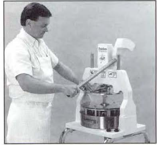
Figure 2: Depress Trip Lever and hold, while pulling Handle down, causing Head Assembly to separate from Trip Lever Plate . . .
