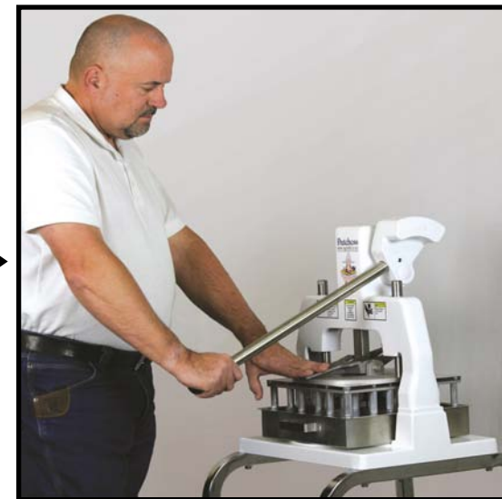
Fig 2: Push downward on the Trip Lever, then pull down on the Operating Handle. This will allow the Head to separate from the Trip Plate.
