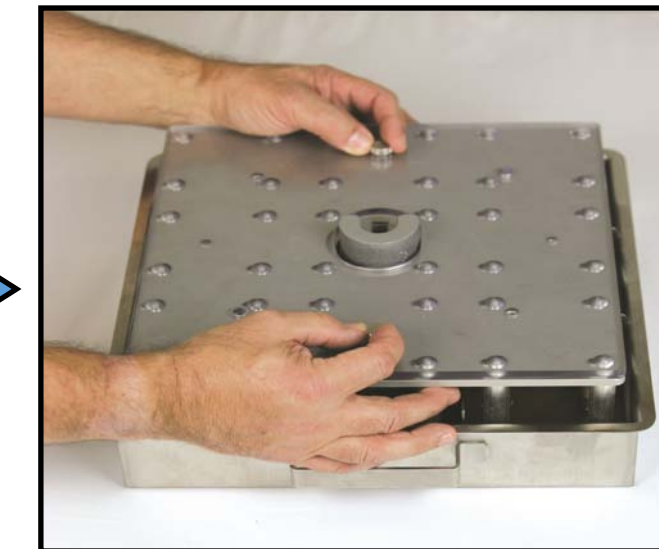
Fig 4: To completely disassemble the Head, begin by removing the two Captured Screws and lifting off the Cover Plate. Note the position of the Captured Screws as they relate to the center of the Head when reassembling.
