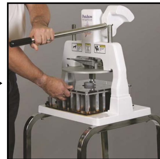
Fig 3: With the Head resting in the Pan (not shown) and the Handle in the down position, pull the Head & Pan towards you until it stops. You can now raise the Handle and remove the Head for cleaning.
