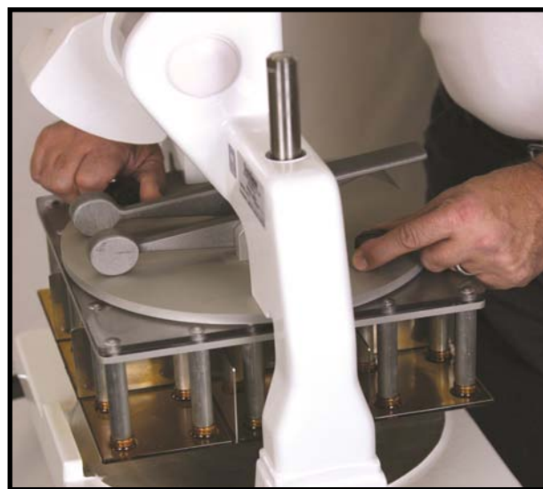
Fig 1: Completely loosen both Black Knobs. Leave pan on the Base for the removal and installation. The pan will assist in the removal and installation.
