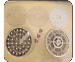
Top L to R: Cover Plate, Locking Plate, Plug Plate Bottom L to R: Pan, Plugs, Divider & Divider Plate
