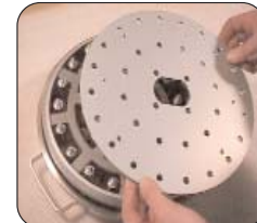
Figure 7: Now lift the Plug Plate, exposing the Divider Assembly.
