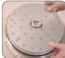
Figure 6: Slide the Locking Plate in the direction to allow Stems to move to the opposite end of the Slots and remove the Locking Plate.
