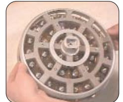
Figure 8: The Divider Assembly may now be removed but need not be disassembled further.
