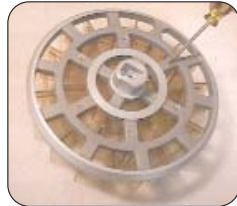
Figure 9: To disassemble the Divider from the Divider Plate, remove the six screws and separate these parts.
