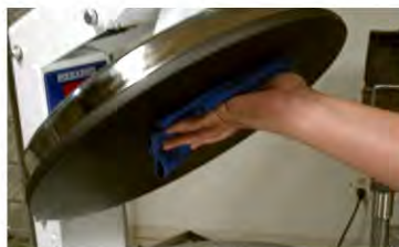
8. Clean upper platen with damp cloth.
