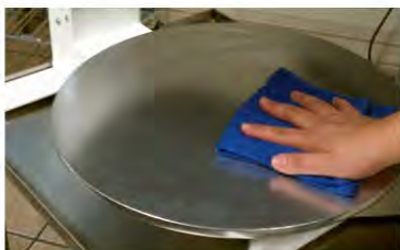
7. Clean lower platen with damp cloth.
