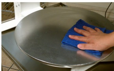
7. Clean lower platen with damp cloth.
