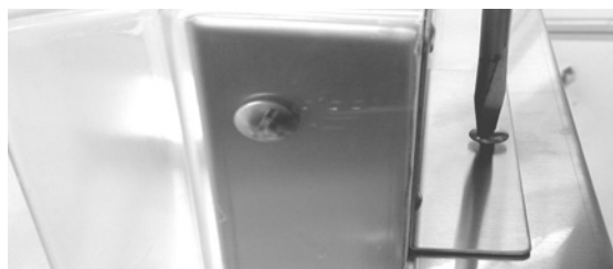
Screw the safety (back of cover)
