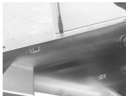
Unscrew the safety (top roller of machine)
