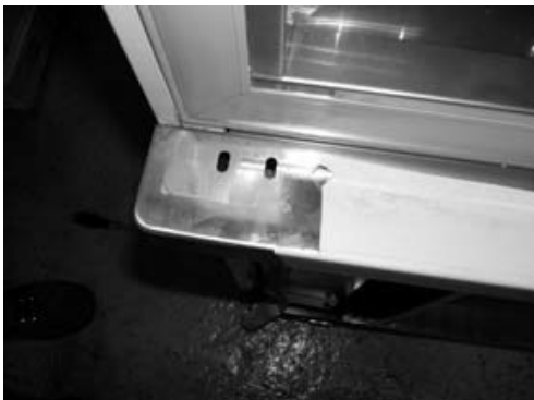
9. Install the door, inserting the top hinge into the prepunched holes, aligning the left lower hinge with the prepunched holes.
