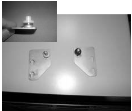
7. Move the black washer and the plastic bushing from the right hinge to the left hinge.
