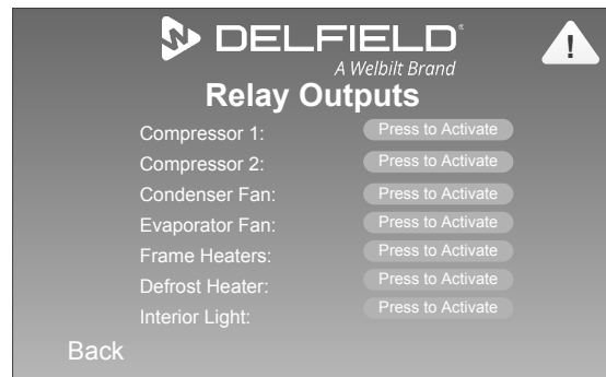
Configuration Screen\Diagnostics\Relay Outputs 1 Section Dual Temperature Unit
