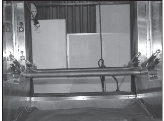
Lifting Plates and 1" Steel Pipes
