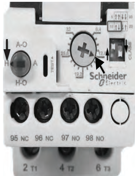
Fig. 32 — 036-2 Units (Size 036, 265V) Overload Settings
