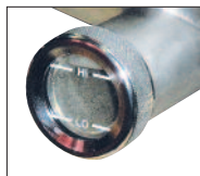
5. Kettle Jacket Water Sight Glass
