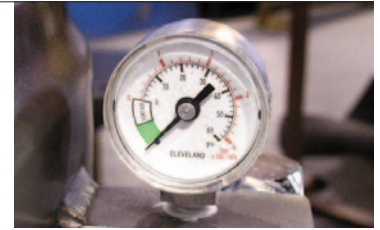
Pressure Gauge in Vacuum.
