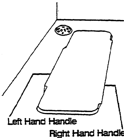
Figure 2-10. Steam Generator Cover in Place
