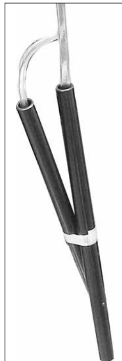
The chemical dispensing pick-up tubes are stowed on the back of the dishwasher.
