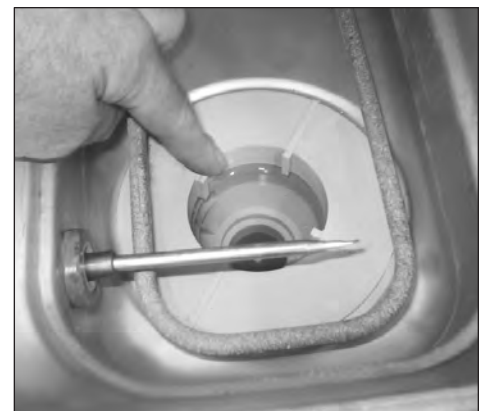
Clean the pump intake screen
