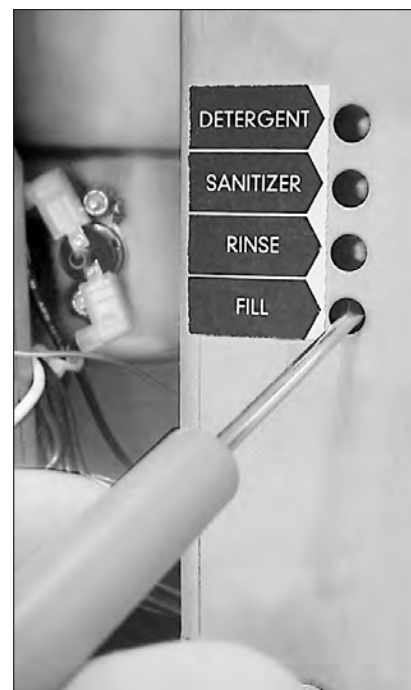
Turning the chemical dispenser adjusting Screws increase or decrease the chemical dispensed.
