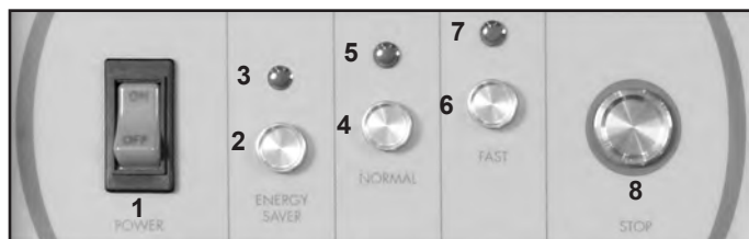
Power Switch is ON, no conveyor speed is selected.
