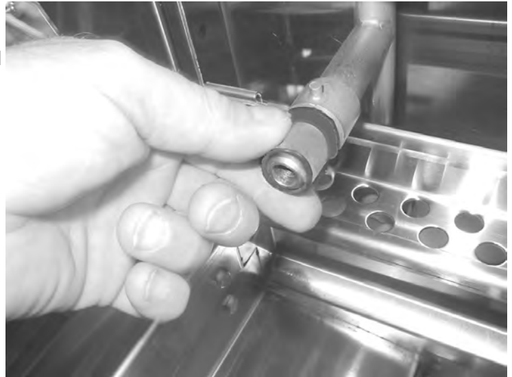
The square-shaped gasket is installed first and the round o-ring is installed second.
