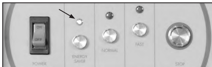
Power Switch is ON, Energy Saver Mode is selected.
