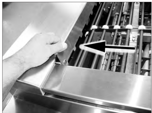
Conveyor Shut-off shelf in the STOP position
