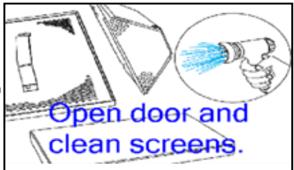
Fig. 85 - Clean scrap screens
