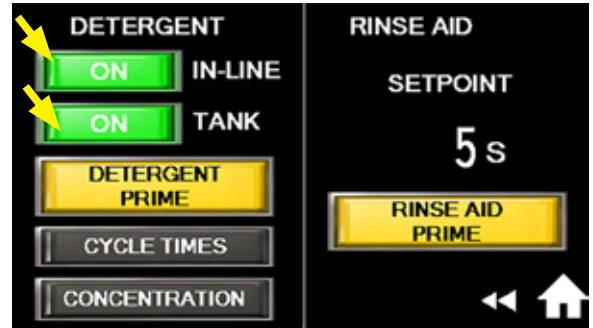
Fig. 36 - In-line and Tank sensor selected.
