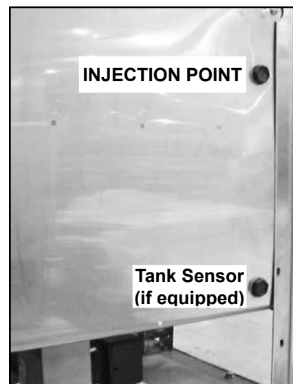
Fig. 18 - Injection and tank sensor (if equipped).
