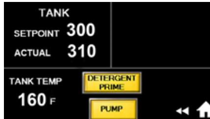
Fig. 39b - Only Tank Sensor ON
