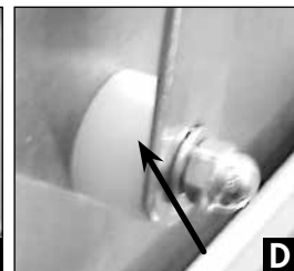
Re-adjust the door springs at the rear of the dishwasher then check that the doors open and close without binding.
