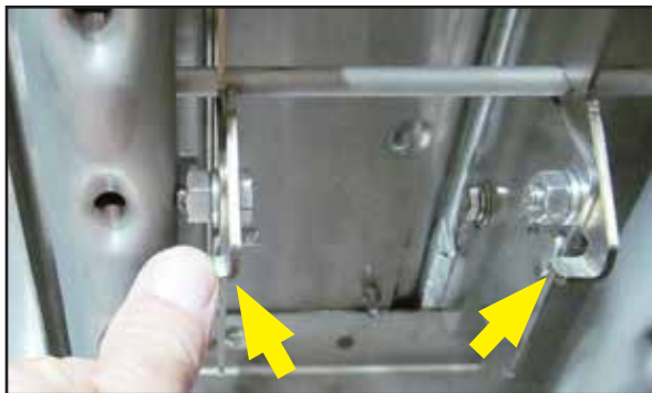
Fig. 64 - Press latches to release upper spray arm.
