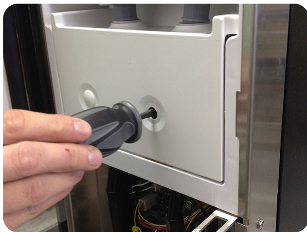
Adjusting Water Flow Using Flat Blade Screwdriver
