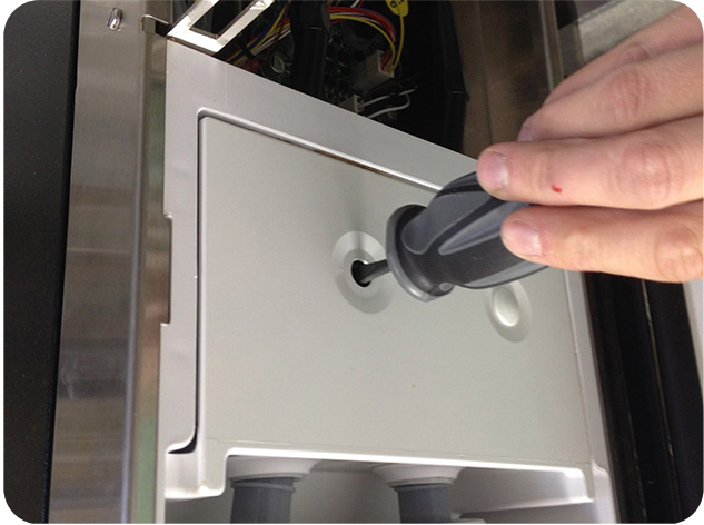
Adjusting Water Flow Using Flat Blade Screwdriver
