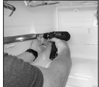
3. Remove the two screws securing the upper rail on one side.
