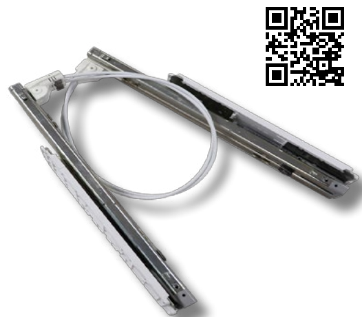
6. Pull both rails and cables out as a complete assembly and replace in reverse order.
