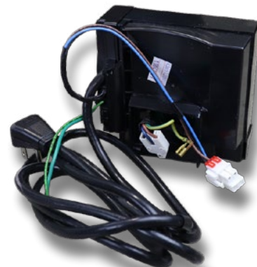
6. Pull the inverter off of the side of the compressor.
