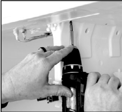
1. Remove the four screws securing the partition to the Freezer ceiling.
