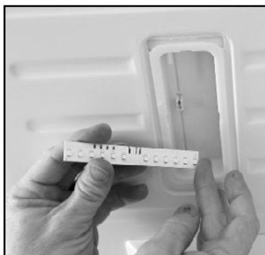
2. Unclip the light board to remove it.
