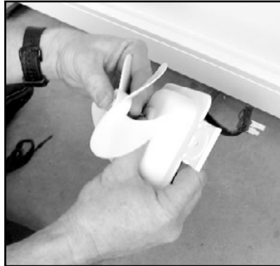
8. Pull the fan blade from the shaft.
