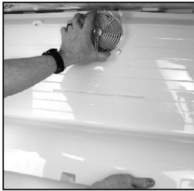
5. Remove the evaporator cover by pulling out on the bottom.
