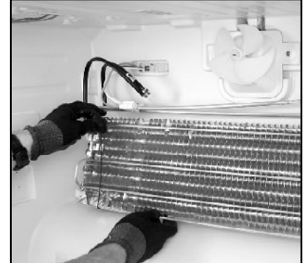
3. Remove the two retaining clips from the front of the evaporator.
