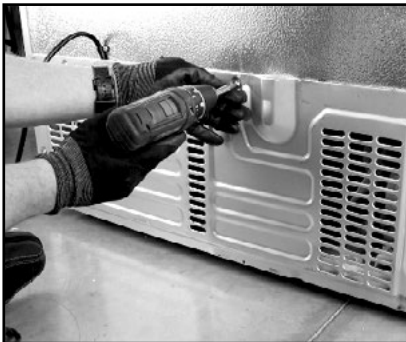
1. Remove the six screws securing the compressor.
