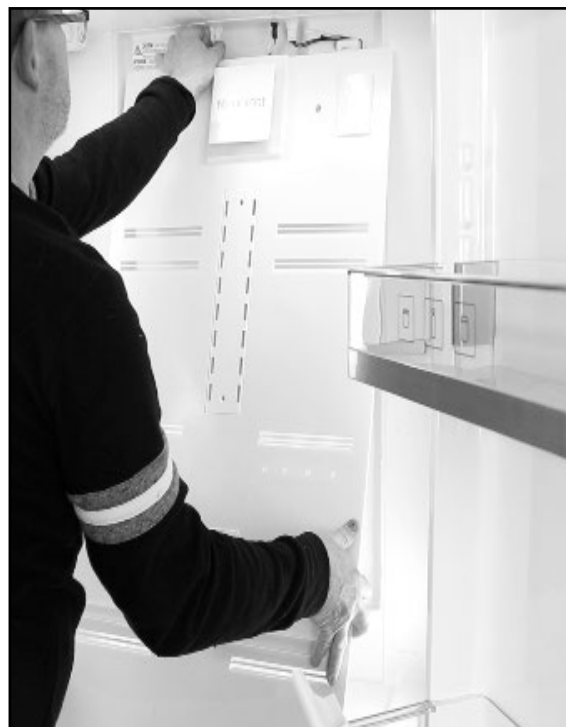
12. Unplug the Fan and Light harnesses and remove the rear panel.
