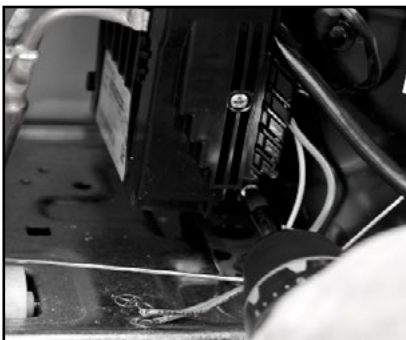
4. Remove the screw securing the inverter to the side of the compressor.
