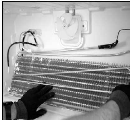
5. Carefully peel the defrost element off of the front of the evaporator.
