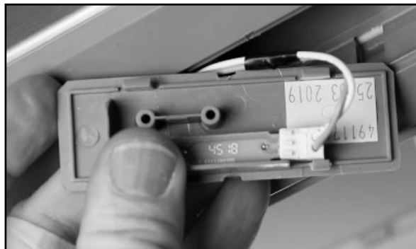
6. Unplug the harness to the Reed Switch.
