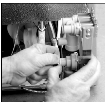
5. Disconnect the hoses from the water valve assembly.
