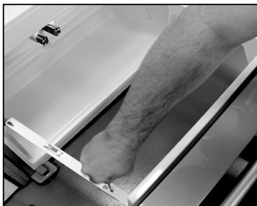
3. Remove the two screws securing the drawer to the rails.
