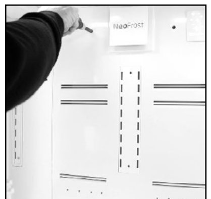
10. Remove the two screws securing the rear panel.
