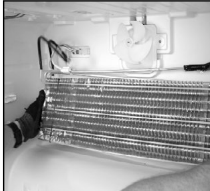
2. Carefully pull forward on the evaporator to unclip it from the rear wall.
