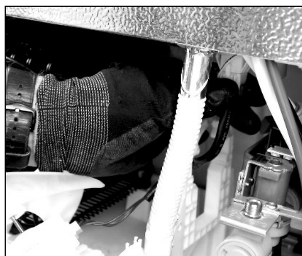
2. Unplug the fan harness from the cabinet and remove the fan. Replace in reverse order.
