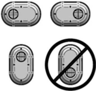
Fig. 11 Approved Installation Orientation
