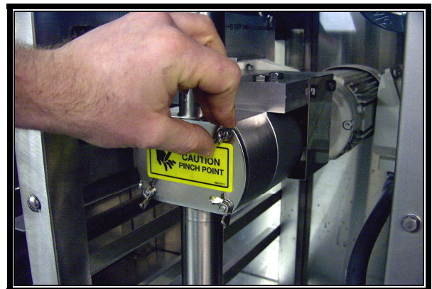
12. Remove the 4 wing nuts from the glaze pump cover.
