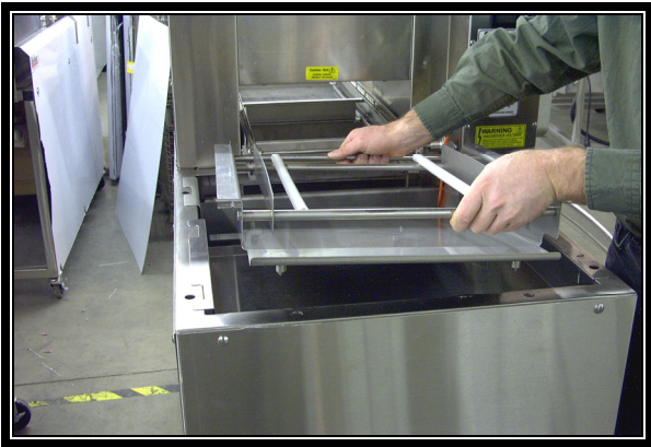
13. Install the drip tray by lining up the locating pins at the outfeed end of the tray.
