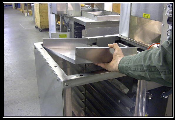
12. Install the outfeed crumb tray.
