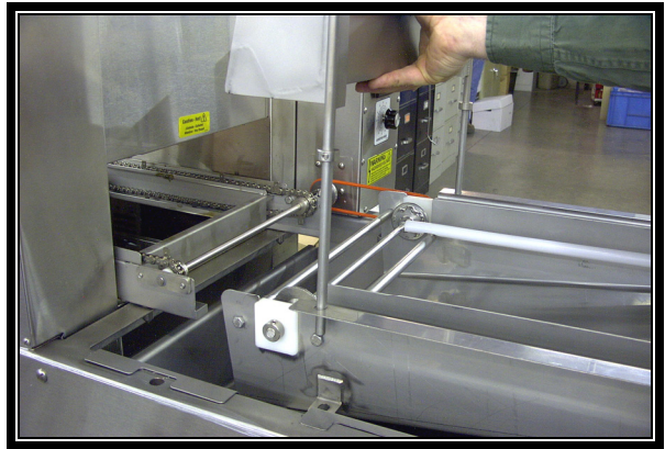
16. Install the glaze trough.
