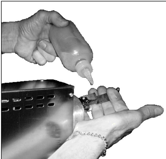
Figure 2-1. Lubricating the Connecting Rod.
