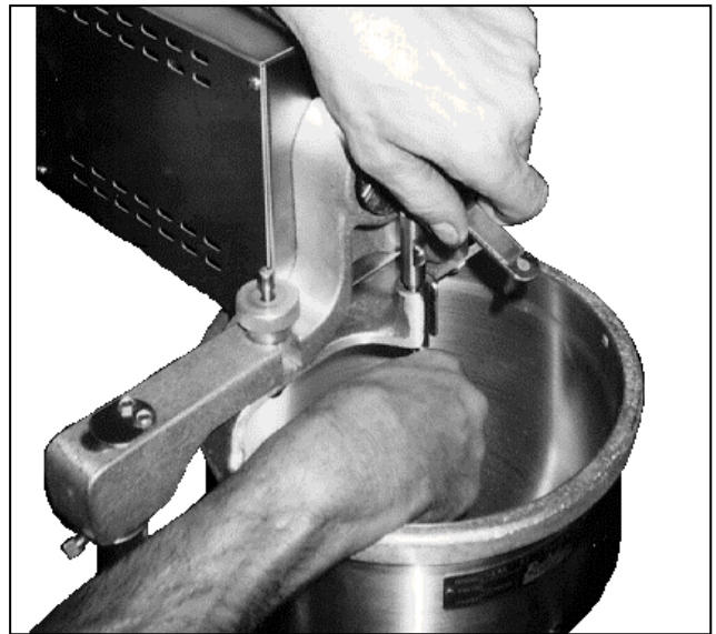
Figure 1-7. Installing the Plunger.
