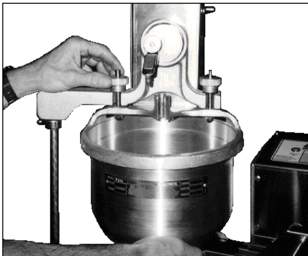
Figure 1-6. Mounting the Hopper.
