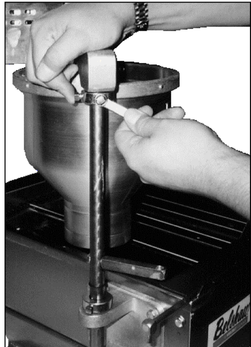
Figure 1-9. Adjusting the Swing of the Hopper.
