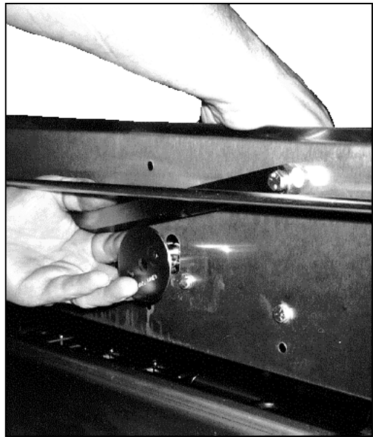
Figure 3 Removing the Turner Cam
