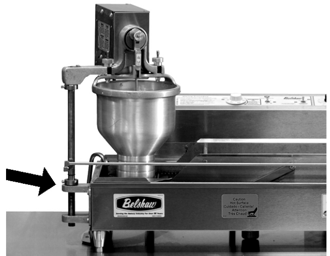
Figure 2-2. Lubricating the swing column.
