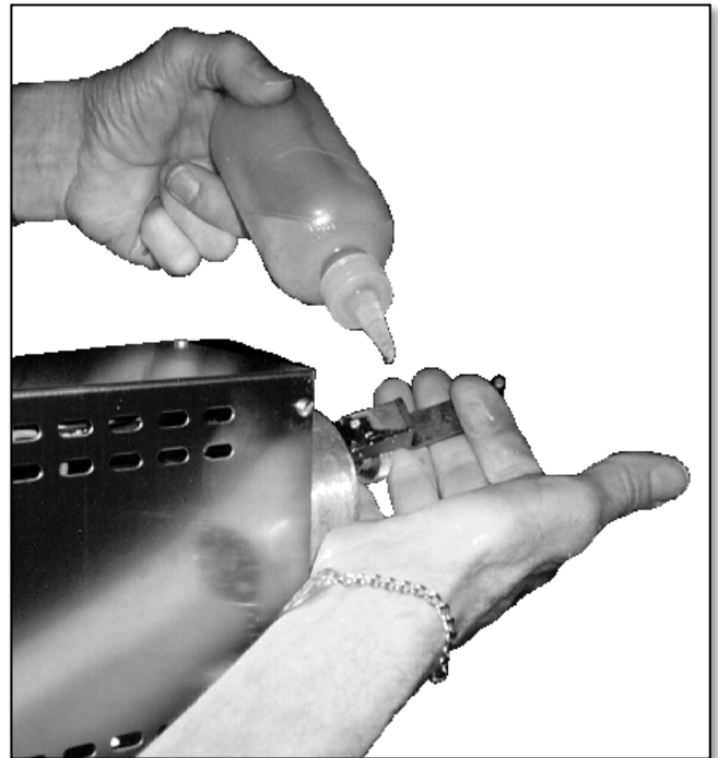
Figure 6 Lubricating the Connecting Rod.
