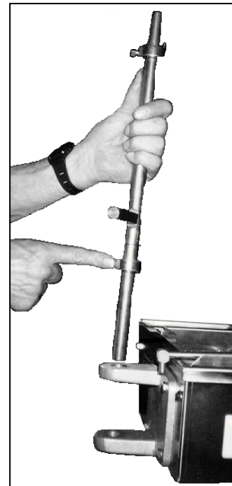
Figure 1-3. Inserting the Swing Column.
