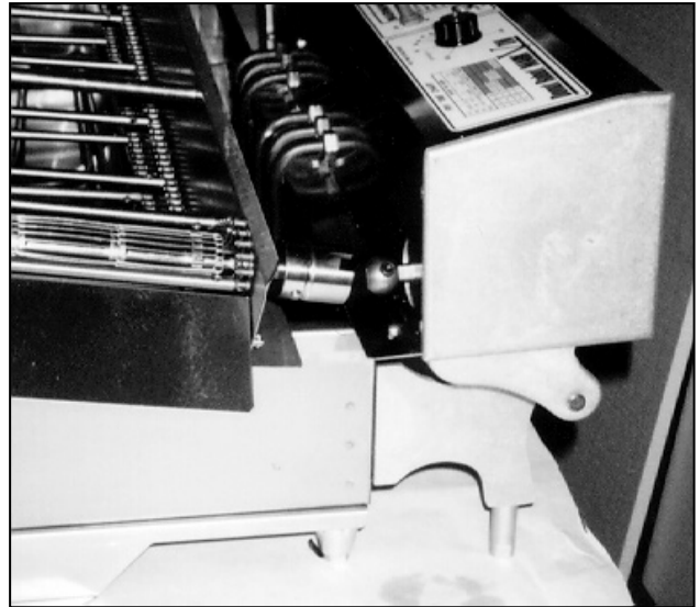
Figure 1-2. Joining the Couplings.
