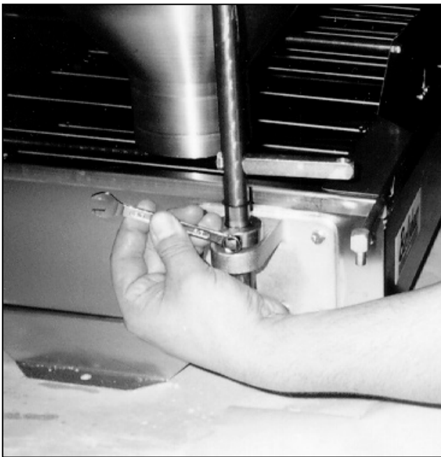
Figure 1-8. Adjusting the Height of the Hopper.
