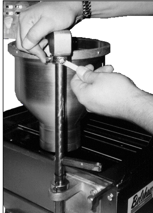
Figure 1-9. Adjusting the Swing of the Hopper.
